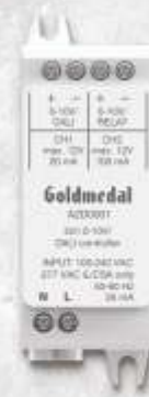
A2D0001 is a BLE-enabled 2 channel 0-10V or DALI controller. It has a universal 100-277V AC input voltage range and can control 2 separate analog channels, 1 Tunable White channel, or one Dali channel.
