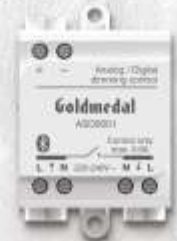
ASD0001 is a BLE-control unit for LED drivers with 0-10V, 1-10V, or DALI dimming interface. The control output can be configured either as analogue 0-10V (and 1-10V) or as a digital standalone DALI control interface.
