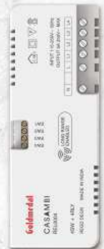
REL0004 is a BLE enabled 4 channel relay with 4 separate inputs to control BLE device on the network. The 4 inputs can be freely programmed to do operations like Dimming, curtains, master functions etc. The device can be used for curtain control also.
